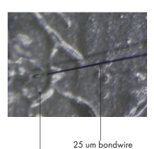
H20 Epotek conductive epoxy
